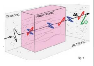
The delay time (Xt) between the arrivals of the fast and the slow shear-waves is proportional to the crack density (or the number of cracks per unit volume).
